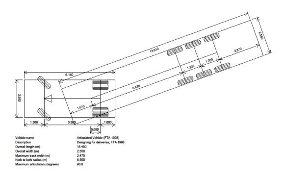
Figure 6.1: FTA Design Articulated Vehicle (Freight Transport Association, 1998)
