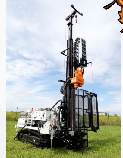
Rotary Drilling Rig that may be utilised for Ground Investigations
