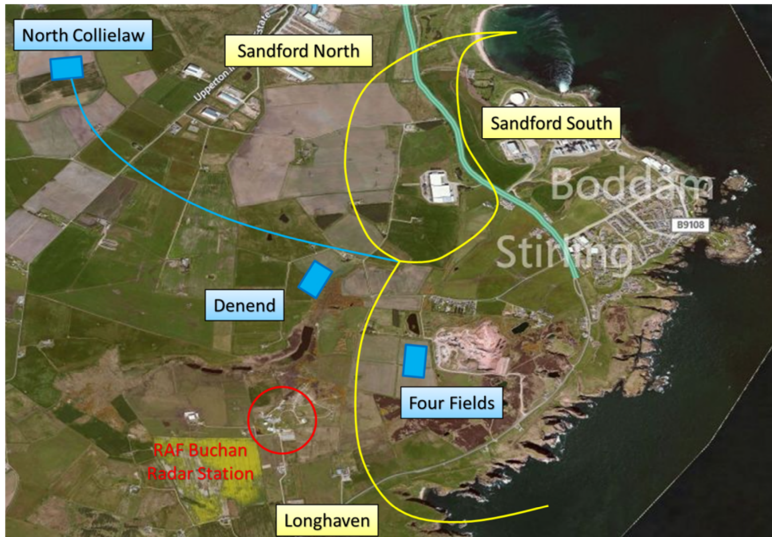
Figure 2.4.2: Converter Station and HVDC Routing Options
